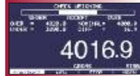
Checkweighing is used when items need to be checked against a pre-set target, after the target weight is set, and over/under parameters are established. Checkweighing is measured as a factor of over the target, under the target, or accept. The display automatically shows the difference in percent and weight.
